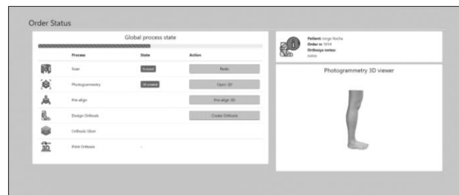
FIGURE III.9 - Workflow from the scanner to the orthotic printout. The user can view all the steps that have been completed or are yet to be done. It's possible to preview the 3D model of the leg or the orthosis.
