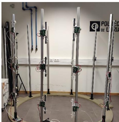
FIGURE 4 - Full Body Scanner structure with 60 cameras
