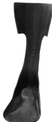
FIGURE III.13 - 3D printed AFO in Nylon 12 material.
