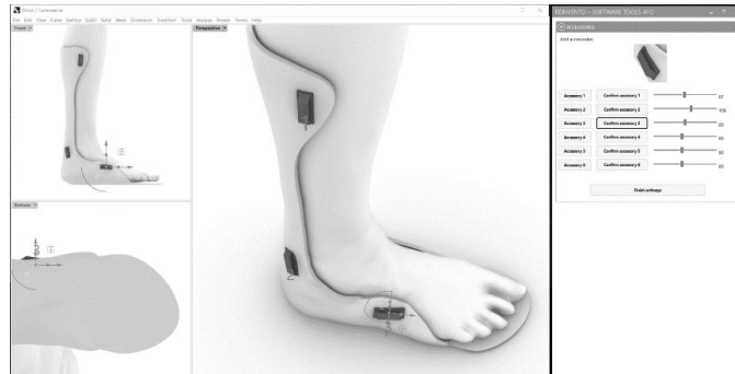
FIGURE III.12 - Design of the final orthosis overlaid on the patient's leg model, with incorporation of eyelets for future placement of velcro straps.
