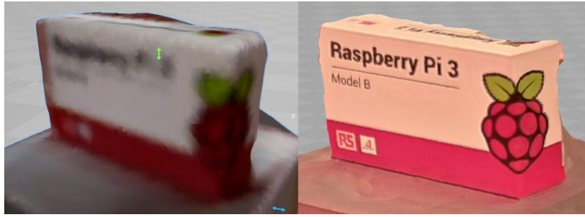
FIGURE 1 - Comparison of textures between the Sense 3D system (left) and Raspberry Pi (right).
