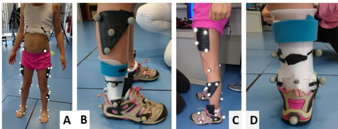
Figure 2-2: Positioning of the retroreflective markers attached to the subjects in several condition. A) Barefoot anterior view; B) AFO-shoe lateral view; C) Shoe Lateral view; D) AFO-shoe posterior view.
